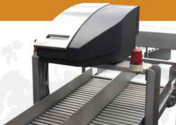
The total printer ESD 104 prints after each batch the respective total label for the box.
