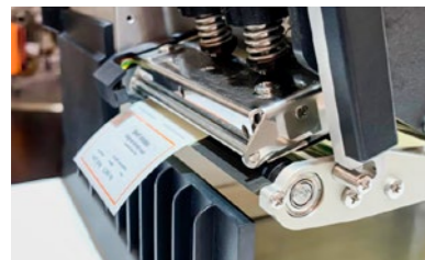
Individual adjustment and balancing of printing force for a perfect label print.
