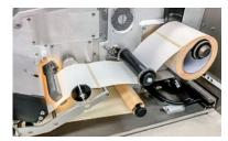
Unique light barrier bar for automatic recognition of different label sizes and label geometries. The ES-M Manual weighing- and labelling system convinces with a unique high-performance printing technology up to 12"/sec.
