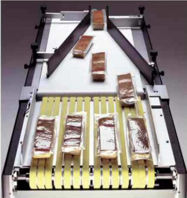
The flexible feed belt control merges up to 6 lanes at the same time
